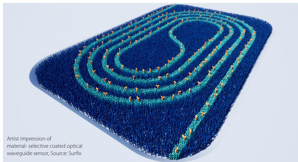
Artist impression of material-selective coated optical waveguide sensor, Source: Surfix
